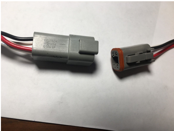
Connector system with crimped pins (Deutsch DT/DTM)
